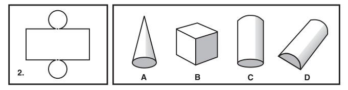
At the left is another drawing of a flat shape. There are no indications on the flat shape to show where it's to be rolled. There are dotted lines where the circles meet the rectangle to show where it's to be folded. Notice that of the four different drawings on the right, only *Object C* can be made by both rolling and folding the flat shape. Therefore, on your answer sheet for Practice Problem 2, the oval under letter  $\underline{\mathbf{C}}$  has been filled in.
